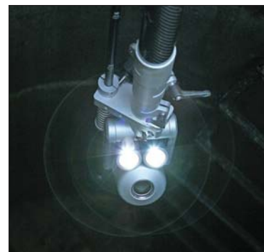
The city's pole-mounted zoom camera enables inspections of pipes from street level.
