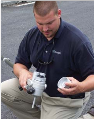
At left, Mike Vislay changes lenses on the camera that features an 18:1 optical zoom, 12:1 digital zoom and 216:1 total zoom. At right, Vislay checks the internal pressure in the camera. The pressurized interior prevents leakage into the camera.
