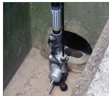
The QuickView Camera, resting on its positioning foot in a storm sewer drop box (left) and at the bottom of a sewer manhole positioned to look upstream.
