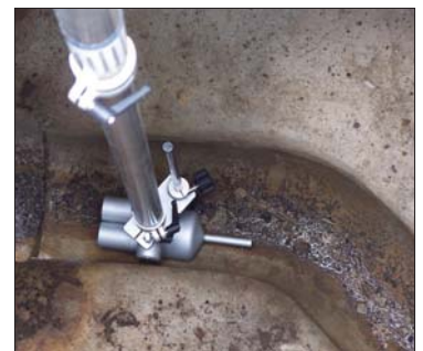
The QuickView Camera, resting on its positioning foot in a storm sewer drop box (left) and at the bottom of a sewer manhole positioned to look upstream.
