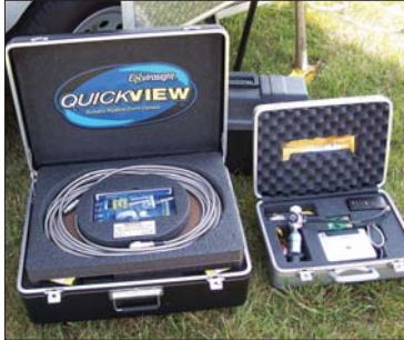
Above, the QuickView camera, cable and control box are transported in the larger case while the smaller case transports the Sony GV ProPack recording system. At right, the QuickView system's video and data information can be sent directly into a wide range of truck-mounted video capture systems.
