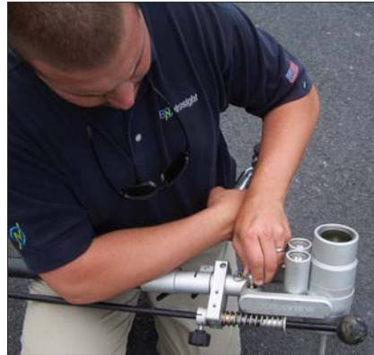
At left, Mike Vislay changes lenses on the camera that features an 18:1 optical zoom, 12:1 digital zoom and 216:1 total zoom. At right, Vislay checks the internal pressure in the camera. The pressurized interior prevents leakage into the camera.
