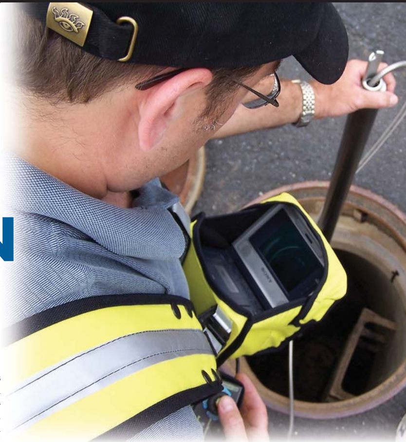
Kelvin Cherrington looks into the view screen of the QuickView camera system from Envirosight LLC as his right thumb controls the focus, zoom and record functions. His left hand steadies the camera, positioned about 12 feet below the surface.
