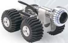
ROVVER 125 chassis with sediment wheels and DigiSewer camera.
