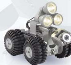
ROVVER 125 chassis with dual large wheels, raise kit, pan/tilt camera and tri-lamps.
